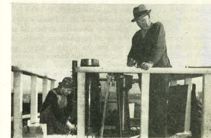
Shipwrights Henry Anderson (standing) and Mac Donell fair up the railing around Monkey Island on the flying bridge.
